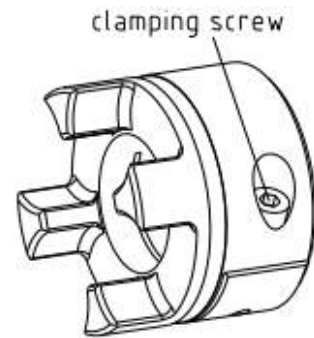
Illustration 20: Assembly of clamping hub
