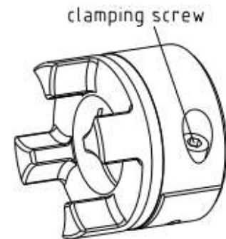
Illustration 20: Assembly of clamping hub
