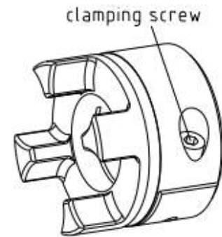
Illustration 20: Assembly of clamping hub
