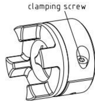
Illustration 20: Assembly of clamping hub
