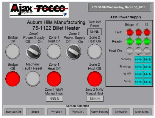
Figure 12-9: Power Supply Screen
