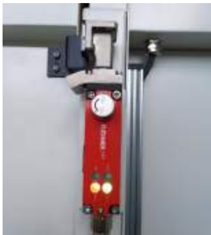
Figure 11 LED indicator of the safety locks
